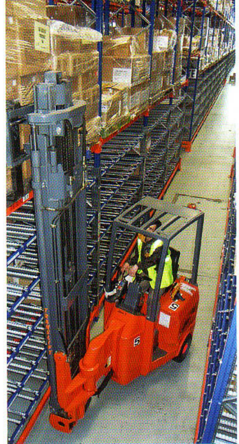
Bendi, a revolutionary counterbalanced, articulating forklift, can work in very narrow spaces.
