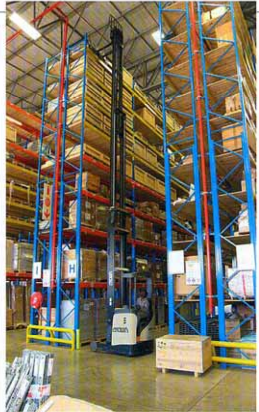
CROWN ESR 5000 REACH TRUCK The truck can reach to a maximum height of 12,5 m
